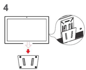
Attach the frame (bracket 1) to the bracket2.
