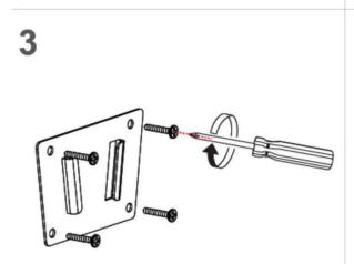
Drill 4 holes on wall, tap the plastic anchors into wall, then attach and screw the bracket2 to the anchors.
