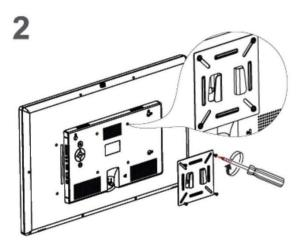
Scew bracket 1 into the back of EOOKE frame.
